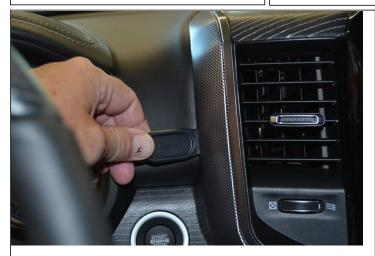
1. Clean the area where the ProClip will attach. insert the gap opener into the seam between the left frame around the left center vent and the padded part of the dash, to widen the gap. (See photo.)
