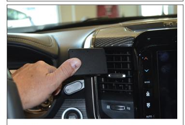
3. Press forward on the left side of the face plate to flex the left attaching edge into the seam above the gap opener.
